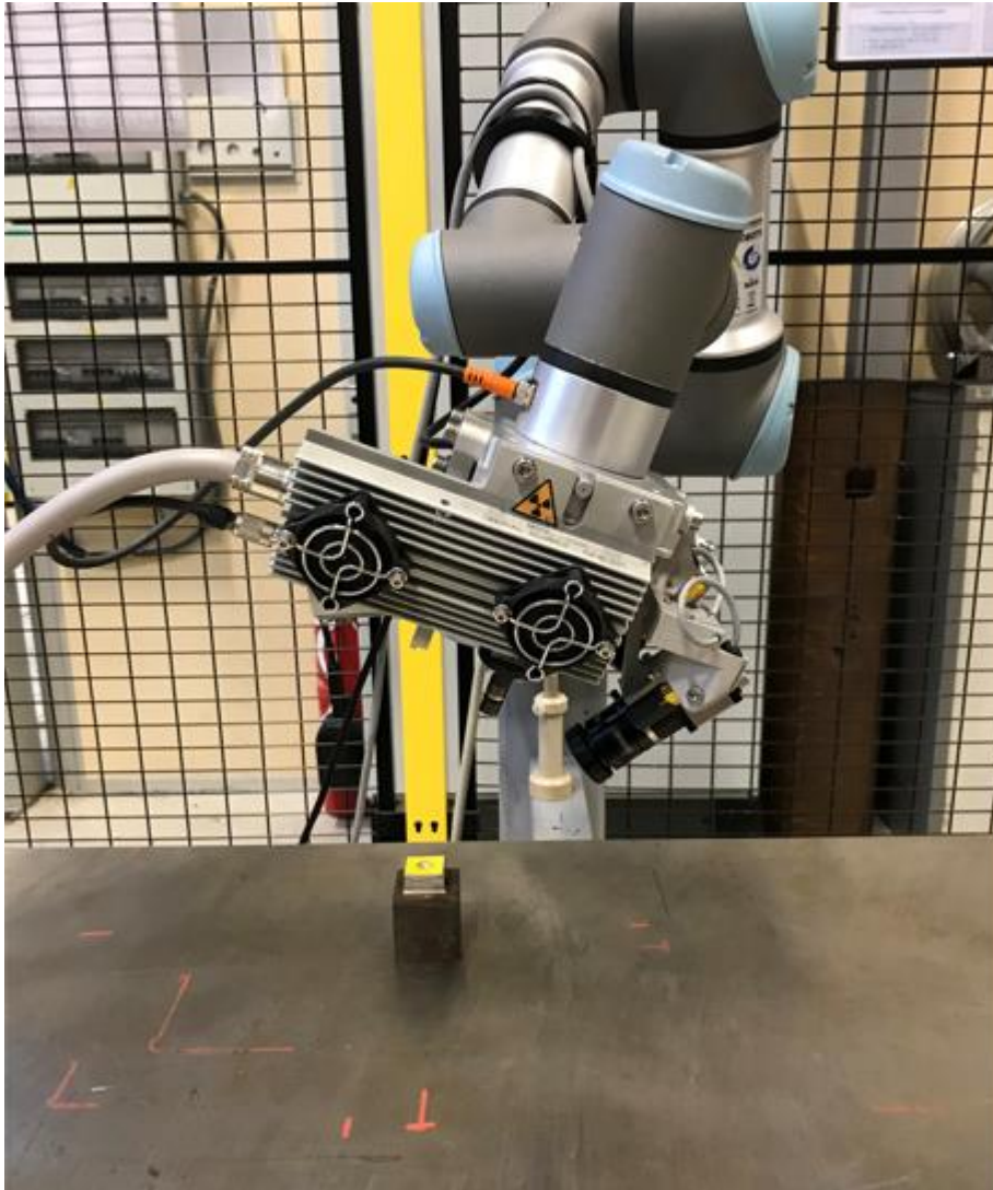
Figure 3 - Illustration of the device used for LXR measurement at CETIM.
