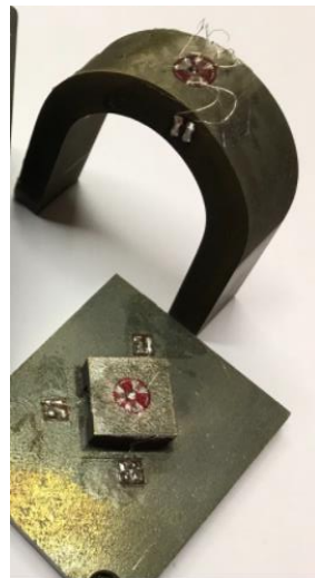
Figure 4 - Localisation of the drilled area on U-bend and on Arches
